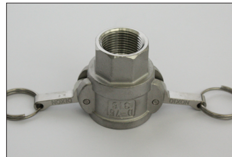
KAMLOK coupler 1 1/2" female, type D, internal thread, stainless steel
