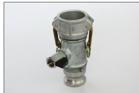
Bypass-valve 10 bar, KAMLOK m/f 1/2", GF T-piece with 1/2" ball valve
